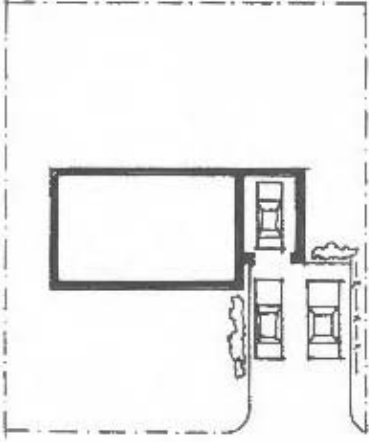
ADDITIONAL PARKING BY WIDENING CURB CUT. This will probably require a permit from your local government.
