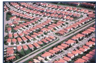
Rooftops, pavements, patios, and driveways contribute to the impervious area in a watershed. This occurs in both urban areas and rural areas being developed.
